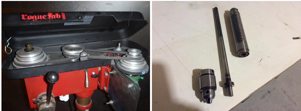
Figure 1: Left - Example belt and pulley system with top of spindle poking out of leftmost pulley. Right - Example chuck, spindle, and quill
