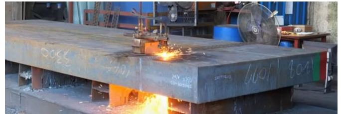
Figure 5. Flame cutting of bar stock for large bearing rings [16]
