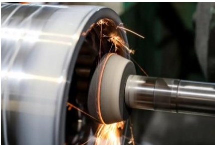
Figure 6. Inner diameter grinding [19]
