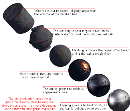
Figure 7. Steps in ball bearing manufacture [19]
